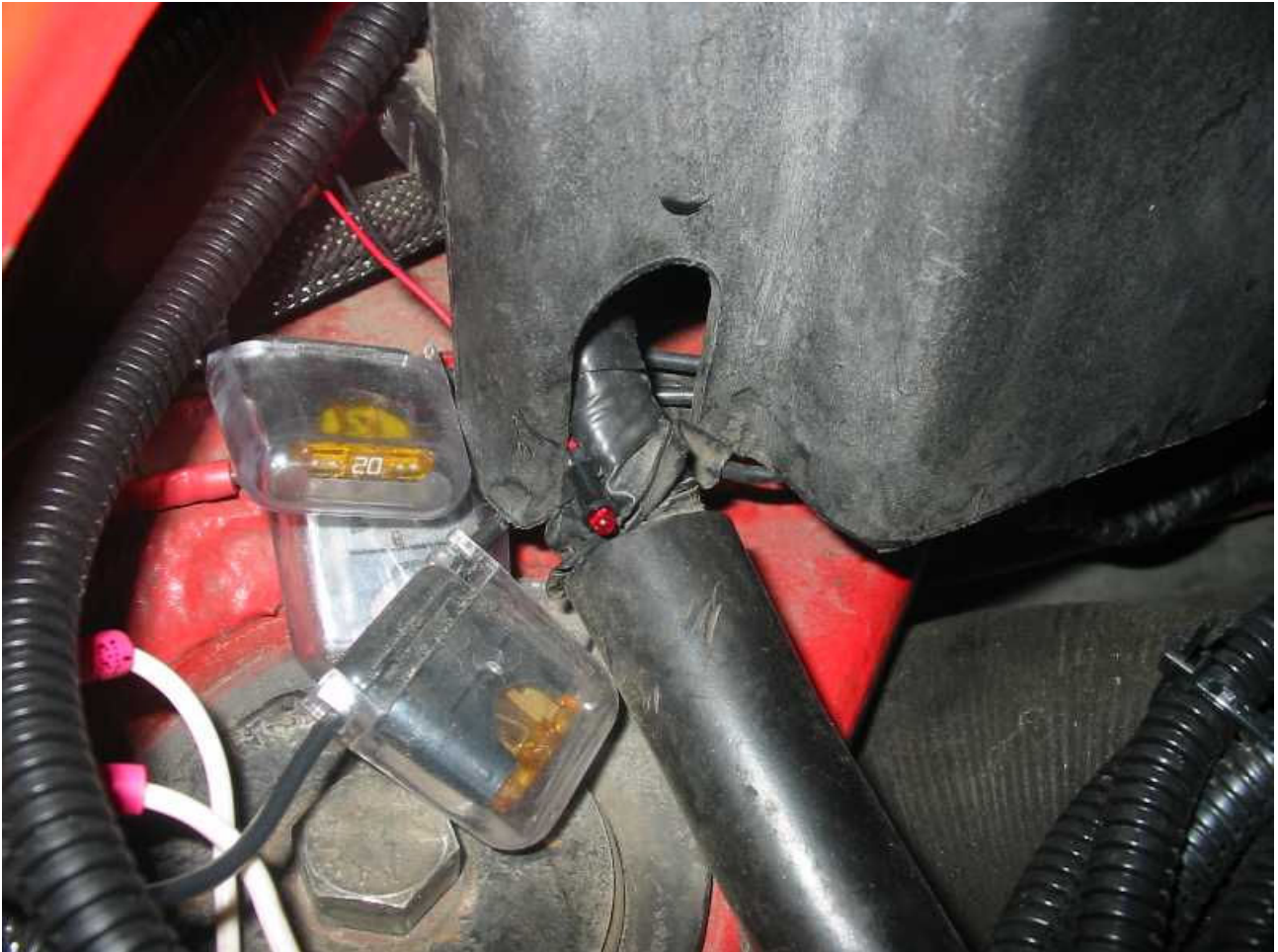
Figure 6: LC-1 LED location
